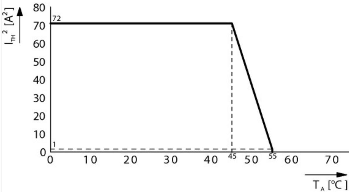
Derating curve - horizontal installation position, without clearance
