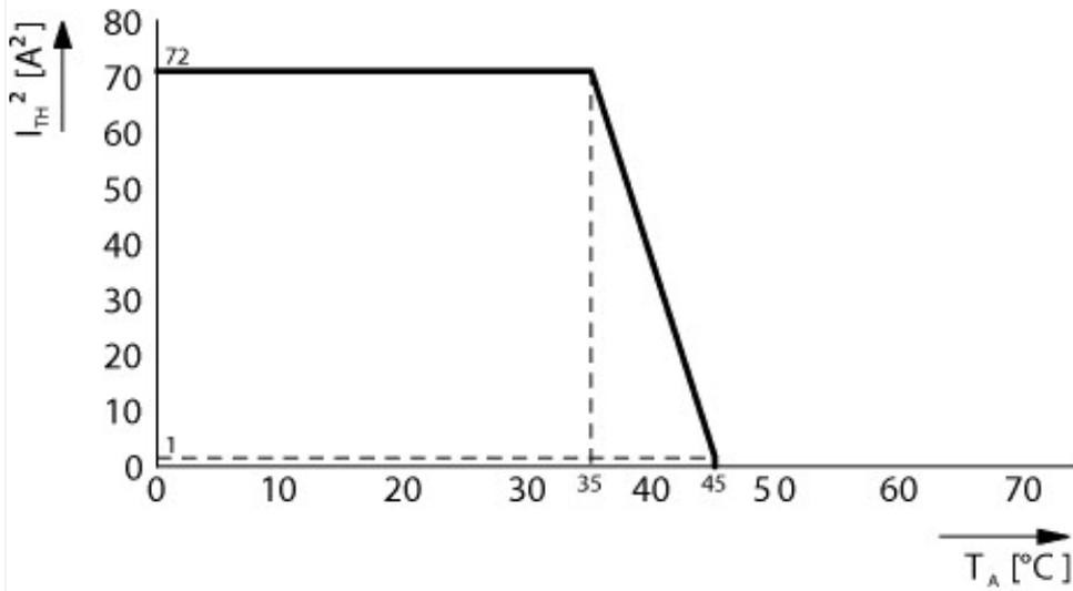
Derating curve - vertical installation position, without clearance
