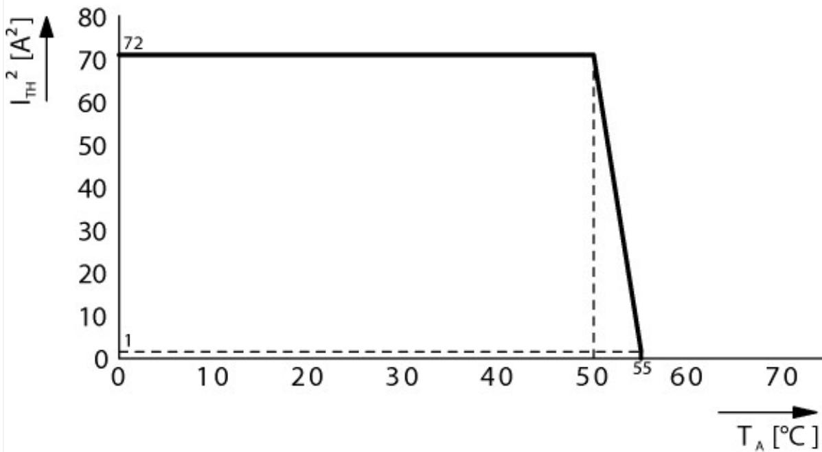
Derating curve - vertical installation position, with clearance
