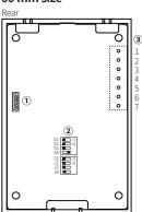
① Expansion connector Using for connecting expansion unit. See 'Connection of Units.'
